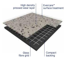
Our PREMIUM COMPACT is made of a >1mm thick, pure inlaid wearlayer pressed under 800 tonnes with no filler, incorporating very densely pressed coloured chips, with a mat finishing and without a transparent wear layer. It offers a T group wear rating and is available in 2 m wide sheet. Its compact backing is calendered, pressed and reinforced with a fiber grid yielding. It offers a 8 dB sound insulation, an indentation resistance of 0.02 mm and a rolling heavy loads easiness.
