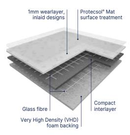
TARALAY MILLENIUM ACOUSTIC is a multilayered vinyl floorcovering available in 2m wide sheet, with a group T wear rating. The product comprises a 1 mm thick coated wear layer, made of pure vinyl, coloured throughout its thickness (no transparent wear layer and no filler). Its complete thickness is 3.4 mm. It contains a Very High Density (VHD) foam backing and is reinforced with 2 fibre glass grids which yields a 17dB sound insulation rating and a resistance to indentation of 0.07 mm.
