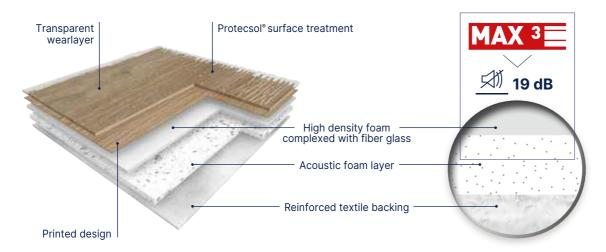
TARALAY LIBERTEX is ideal for fast track installation or renovations in commercial buildings. It is a multi-layered vinyl floorcovering with a printed design protected by a 0.70 mm thick transparent wear layer. The product features a high density foam complexed with fiber glass, an acoustic foam layer and a reinforced textile backing. It offers 19 dB sound insulation.
