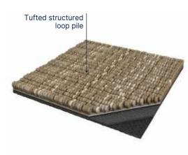
**Armonia 620** is a decorative, reliable, hardwearing textile floor covering. It consists in a tufted 50 × 50 cm structured loop pile carpet tile with a 3,2 mm pile height. The overall thickness is 6,5 mm with 620 pile weight.
