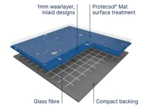
TARALAY MILLENIUM COMPACT is a multilayered vinyl floor covering available in 2m wide sheet, with a group T wear rating. The product comprises a 1 mm thick coated wear layer, made of pure vinyl, coloured throughout its thickness (no transparent wear layer and no filler). Its complete thickness is 2 mm. It is reinforced with a fibre glass grid for a better dimensional stability. The construction of the product yields a 8dB sound insulation rating and a resistance to indentation of 0.03 mm.
