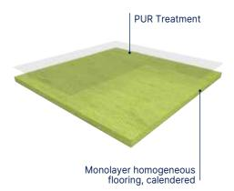
MIPOLAM CLASSIC 1.5 mm is a flexible homogeneous calendered compacted floorcovering in tiles or sheets, with directional design, colour dyed as a raw mixture to ensure even colour throughout the thickness of 1.5 mm and a **weight of ≤ 2520 g**. Its surface is densely compacted for improved wear and ease of maintenance.
