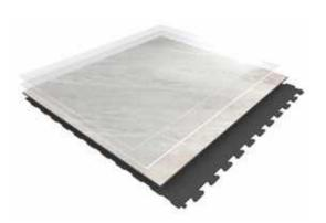
**Design Tile** is a synthetic, decorative, flexible, antistatic, abrasion group T floor covering. It consists in a multilayered tile with a 0,70 mm thick transparent wear layer and a printed film on an injected molded backing. The overall thickness is 7,8 mm.
