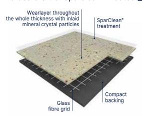
TARASAFE ULTRA is a hardwearing safety flooring collection that comprises of a PVC wear layer and deeply inlaid mineral crystal particles (patented) and coloured chips for a decorative design. It is suitable for heavy traffic areas and is ideal for hardworking contract applications. It delivers Safety in Numbers, with a PTV >36+ slip resistance (Dry & Wet), a R10 wet slip resistance rating and >20 Rtm/Rz surface roughness in accordance with HSE quidelines.
