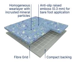
TARASAFE ULTRA H2O is a slip resistant vinyl floorcovering, wearlayer throughout the whole thickness and deeply inlaid mineral particles and coloured chips for a decorative design together with a raised emboss for better slip resistance.
