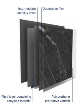
**MURAL REVELA** is a rigid vinyl wall covering which has a thickness of 5mm for an extended durability. It is available in 2 formats of  $65 \times 37,5$ cm for tiles or  $260 \times 90$ cm /  $260 \times 120$ cm for panels. It is intended for indoor use.
