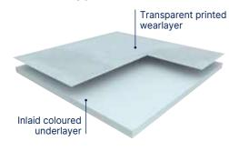
MURAL CALYPSO is a multilayered wall covering in 2 m width roll and with a B-s2,d0 fire classification according to EN 13501. It is hot welded with CR40 welding rods for a perfect water tightness. It is made of a printed transparent wear layer and a coloured under layer for a better aspect of the welding. This layer comprises up to 30% of recycled products.
