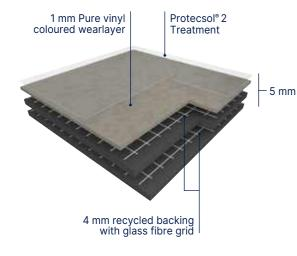
ATTRACTION® is a semi-flexible tile constructed by compacting, at high temperature and over 3000 T, a 4 mm recycled backing and a 1 mm Pure vinyl wear layer. This wear layer is incorporating very densely pressed coloured chips, with a mat finishing and without a transparent wear layer. The product comprises a compact backing which is pressed and reinforced with two glass fibre grids.
