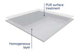
MURAL CLUB is a homogeneous wall covering in 2 m width roll and with a B-s2,d0 fire classification. It is designed to be a permanent wall covering. It is hot welded with CR40 welding rods for better hygiene. It is made of calendered layer with colour throughout the whole thickness for an nicer aspect of the welding. This layer comprises at least 10% of recycled products. It does not contain any CMR 1 & 2 component and is 100% compliant with REACH. It is 100% recyclable.
