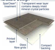
**TARASAFE COMPACT DESIGN** is a slip resistant vinyl floorcovering in sheet, which transparent wear layer contains deeply inlaid mineral crystal particles for durable shod (R10 according to DIN 51130) and barefoot (B according to DIN 51097) antislip performances. It is available in 6 realistic wood or mineral designs thank to a printed layer.
