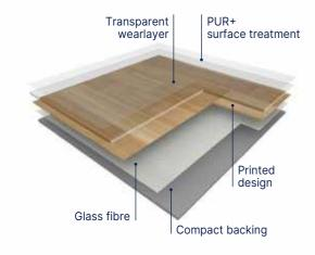
**NEROK** is a multilayered vinyl floor covering available in 2m and 4m wide sheet, with a group T wear rating.
