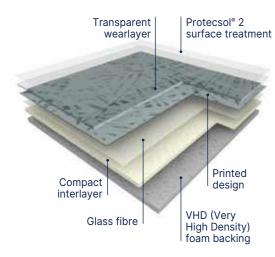
TARALAY IMPRESSION ACOUSTIC 0,65 is a multi-layered vinyl floorcovering, integrating a Very High Density foam backing, reinforced with a fiber glass and a printed design. It's available in 2 m wide sheet, with a group T wear rating.
