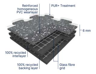
**GTI® Pure** is a multi-layered interlocking looselay vinyl tile with polyurethane treatment **(PUR+)**, 6 mm thick with a dovetail joint for the **Connect** configuration.
