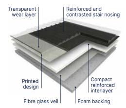
TARASTEP PRO is an heterogenous, sound-absorbing solution with reinforced layer and transparent wearlayer, used to recover indoor stairs in a single element.
