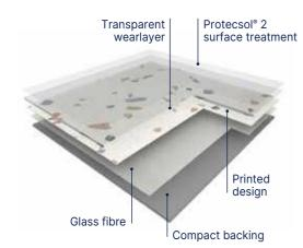
**TARALAY IMPRESSION COMPACT** 0,7 is a multi-layered vinyl floorcovering, integrating a fiber glass and a printed design. It's available in 2 m wide sheet, with a group T wear rating. Total width of the product is 2 mm, including a transparent wear layer of 0.70 mm thick. It offers 8 dB sound insulation and an indentation resistance of ca. 0.03 mm. Its dimensional stability performs down to 0,08% (average measure).
