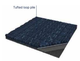
**Armonia 400** is a decorative, reliable, hardwearing textile floor covering. It consists in a tufted  $50 \times 50$  cm loop pile carpet tile with a 2,3 mm pile height. The overall thickness is 5,3 mm with 400 pile weight.
